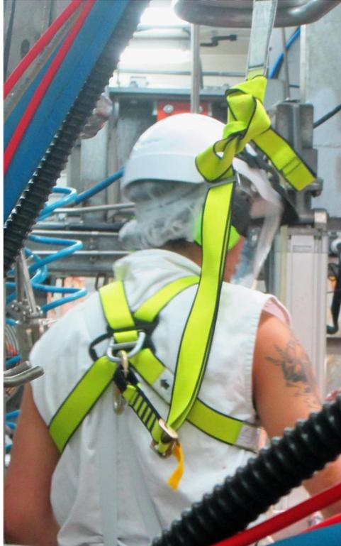
A rail at least 900mm high, with gaps no more than 470mm. Where this cannot be fitted because, for example, working down the carcass in production, then consideration should be given to a fall restraint or fall arrest harness. Toe guards on the edges should be considered.
