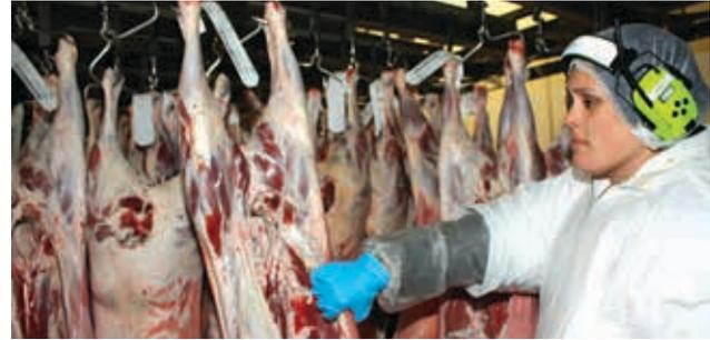
Carcasses are chilled under carefully controlled conditions
